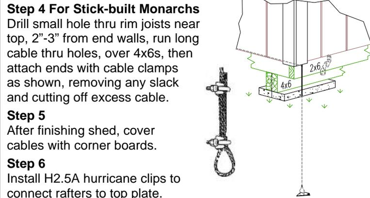
**Hurricane Clips** are also included with our Anchor Kits, to attach the rafters to the top plates of the walls. We use Simpson Strongtie H2.5A, which have a rating of 480 lbs of uplift load each. Stick-built Monarchs come standard with hurricane clips.
